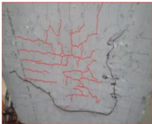
Figure 4: Crack pattern and mode of failure S1-0
