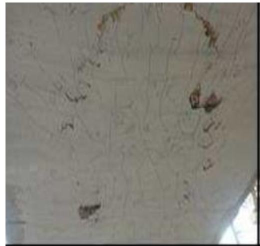
Figure 5: Crack pattern and mode of failure S3-35
