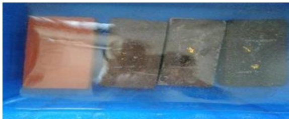
Figure 4: Immersed bricks in water for 24hrs
