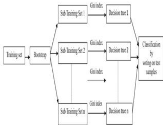
Figure 4: RF classification algorithm Flowchart
