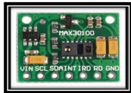
Figure 3: max 30100 pulse oximeter
