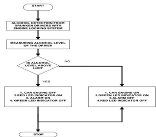
Figure 6: Flow Chart of Alcohol Sensor
