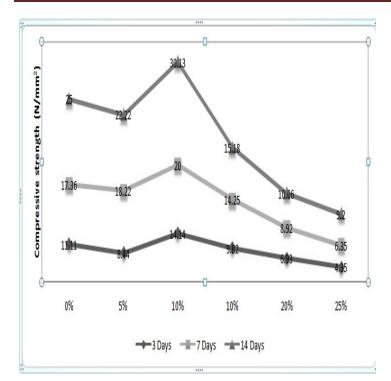
Figure3: Effect of RHA on 3, 7 & 14 days compressive strength
