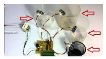
As shown in Fig: 3.2.2 The Garbage Monitoring System will look like that. Ultrasonic sensors are used to detect the height of the garbage bins the ultrasonic sensor is interfaced with Arduino to get the readings and according to
