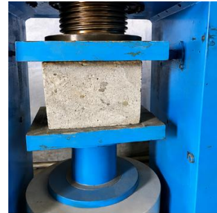
Figure 7: Concrete Cube under Load
