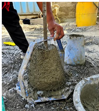
Figure 6: Slump of Replacement Concrete
