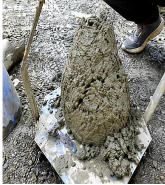
Figure 5: Slump of Conventional Concrete
